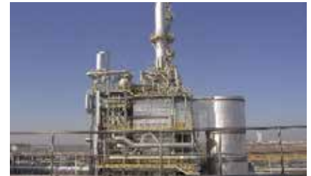
Caojing/CN, 4.500 kg/h liquid, 327.000 Nm 3 /h Off-Gas
